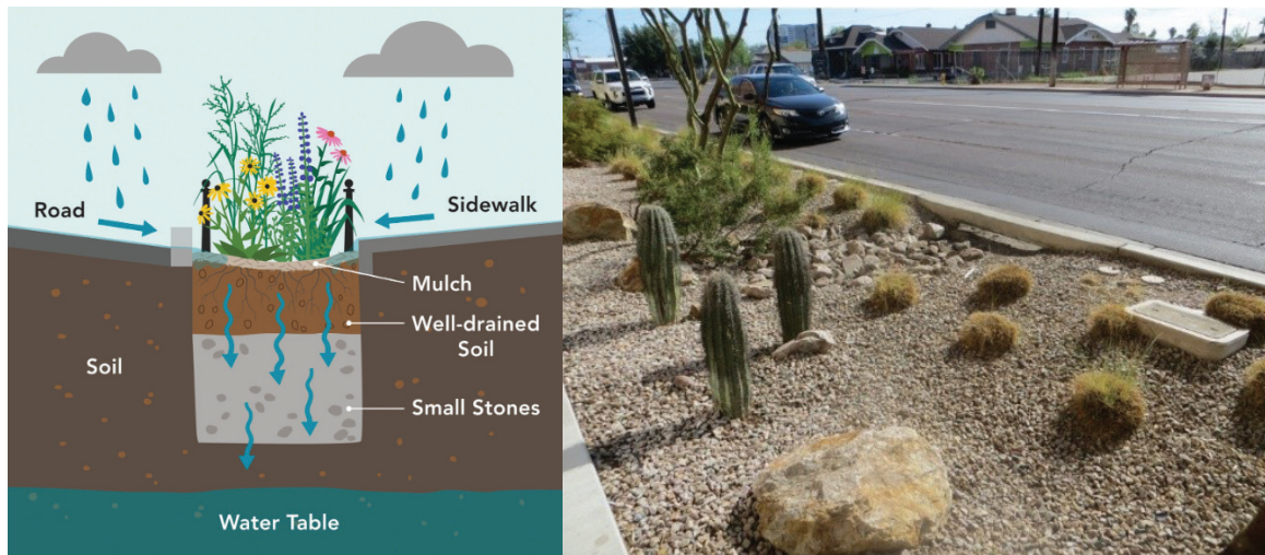
Figure 22: A schematic representation of the structure (left; Tait, 2014 ), and a photograph of a bioswale (right; Coe & Van Loo Consultants, Inc., 2018 ).
